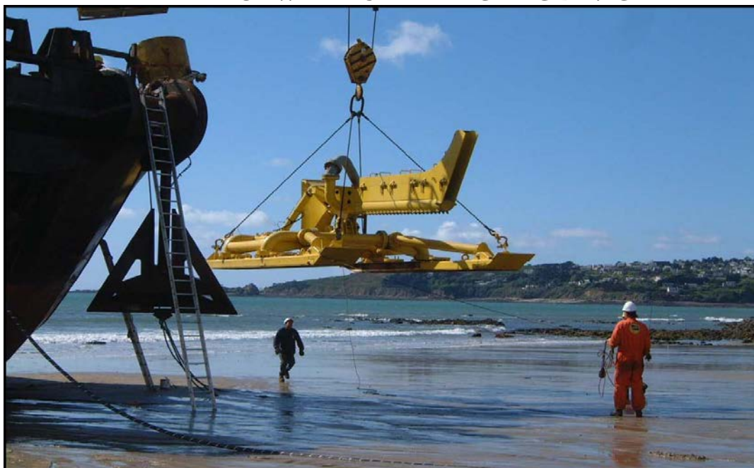
FIGURE 2-13 EXAMPLE OF WATER JET TRENCHING DEVICE
